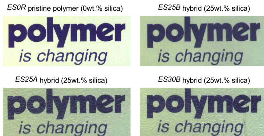
Fig. 1. Photographs of the pristine epoxy polymer and different epoxy–silica hybrids signifying the optical transparency or opaqueness of thin films.
